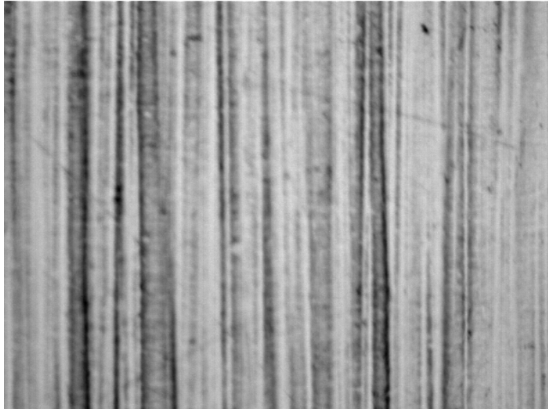
Figure 1. Image of the roughness standards comparator with R_a=0.2 . Image size is 160 \times 130 \mu\text{m} .
