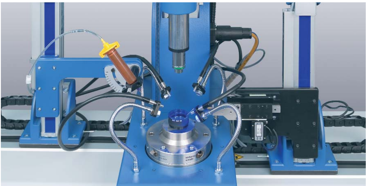
Detailed view of OptiCentric® Bonding Station. Left: Dispenser stage, Right: Piezo manipulator stage, Center: OptiCentric® MOT system featuring air bearing stage and electronic autocollimator
