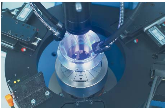
Automated assembly of infrared optics
