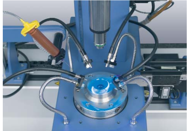
UV curing of a centered lens with four light guides. Left: Dispenser, Right: Piezo manipulator, Top: autocollimator with microscope objective
