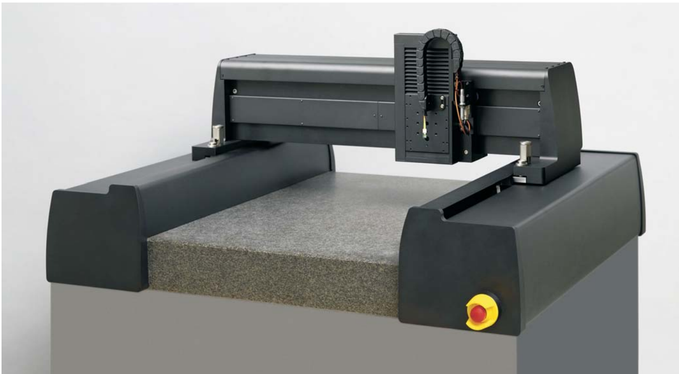
Airbearing gantry LLP 782350-600 with ball screw z-axis
